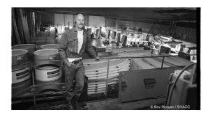
∞ They came up with a way to mold polyurethane foam into a surfboard shape, and Hobie started to market these new lightweight boards in the mid~to late~1950s.
